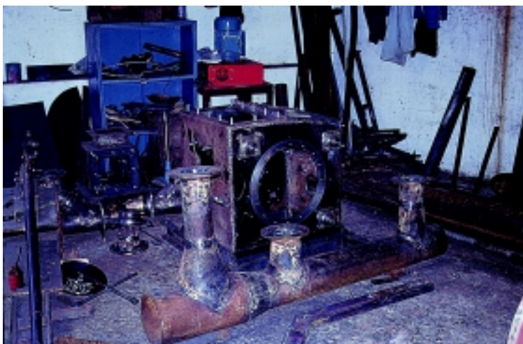
A turbine being manufactured at Kathmandu Metal Industries
